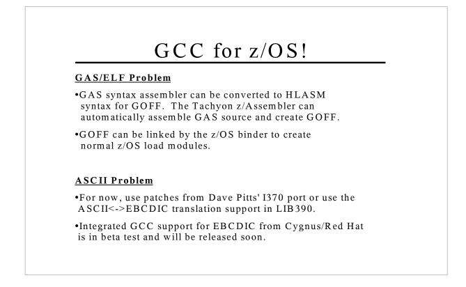
The Tachyon z/Assembler can be used for free when used to assemble the output of the GCC compiler. The free version can generate either GOFF (31-bit) or ELF (31-bit or 64-bit) object files from GNU assembler source. The free version of the Tachyon z/Assembler can be downloaded from the Tachyon Software web site at <a href="http://www.tachyonsoft.com">http://www.tachyonsoft.com</a>
