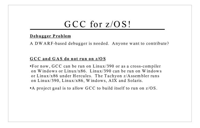
Using cross-platform development tools like GCC and the Tachyon z/Assembler, you can build programs on one platform to be executed on another. For instance, you can build the object files for a program on Linux and then upload them to z/OS where they can be bound into Program Objects or Load Modules and executed.
