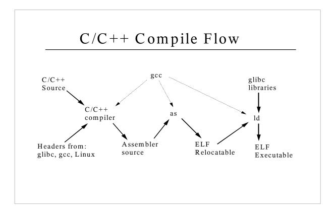
gcc is the controller program for the compile process. Unless told to do otherwise, it will invoke the  $C/C^{++}$  preprocessor,  $C/C^{++}$  compiler, the assembler (as) and the linker (ld).
