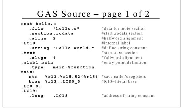
This is the 31-bit GNU assembler code produced by GCC 3.02 for Linux for S/390. The comments generated by GCC are omitted. The comments to the right of the GNU assembler code were added by hand.
